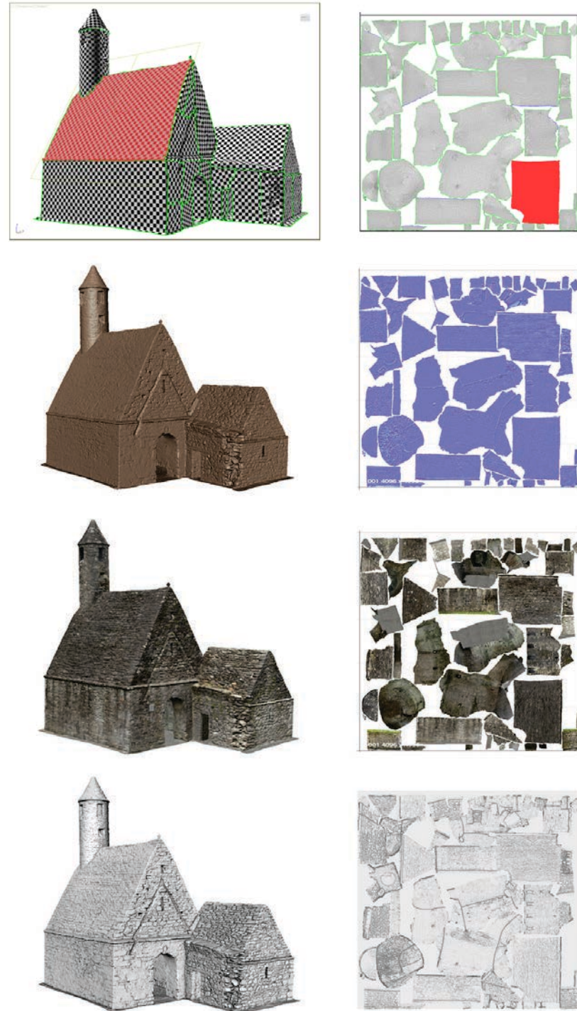
DIAGRAM ILLUSTRATING THE DIFFERENT TEXTURE MAPS WHICH CAN BE EMPLOYED TO ENHANCE THE DISPLAY OF A LIGHTWEIGHT 3D MODEL. FROM TOP: UV MAP, NORMAL MAP, IMAGE MAP AND AMBIENT OCCLUSION MAP (DISCOVERY PROGRAMME)
