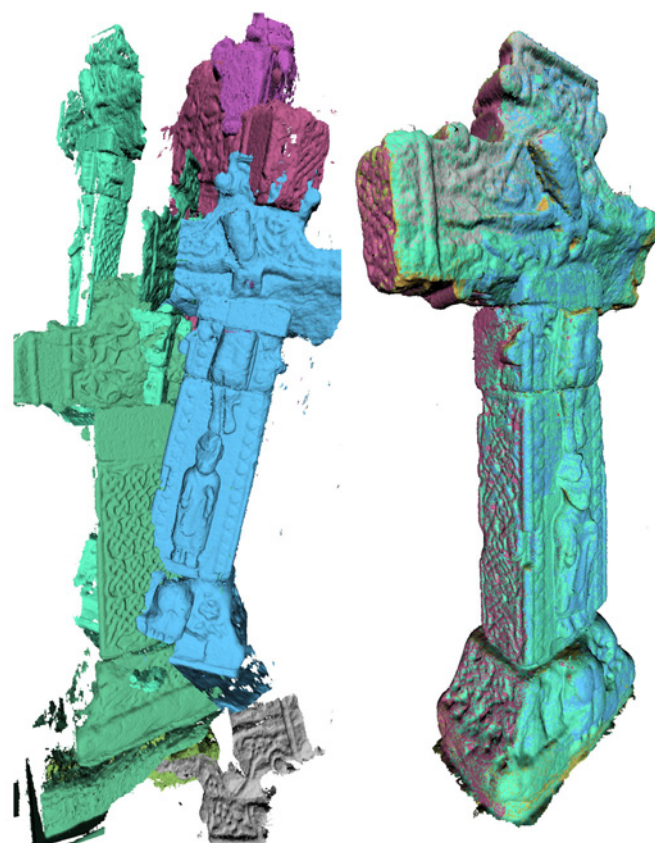
IMAGE OF THE PRE AND POST ALIGNED INDIVIDUAL SCANS WITHIN ARTEC STUDIO
