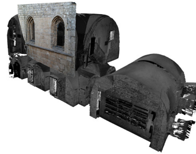
3D MODEL OF THE CENACLE COMPLEX FACADE - INTEGRATION OF STRUCTURE-FROM-MOTION MODEL WITH TERRESTRIAL LASER SCANNING
