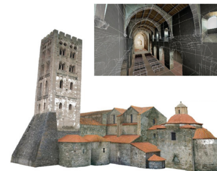
3D MODELING OF THE EXTERIOR AND THE INTERIOR OF THE ABBEY INCLUDING REALITY-BASED TEXTURING
