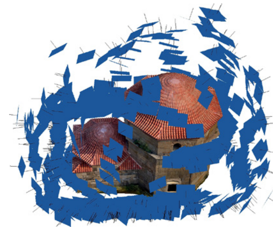
SPATIAL DISTRIBUTION OF A SET OF IMAGE SEQUENCES USED FOR THE GENERATION OF THE SFM-BASED 3D MODEL
